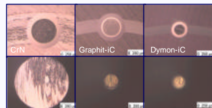
Fig. 5: Taper cross section of coating wear track and wear scar on chrome steel ball following testing of coatings in air under an applied load of 40 N after a sliding distance of 720 m
